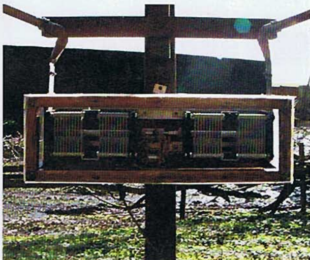
PHOTO 2: Detail of the tuning capacitance mechanism.
